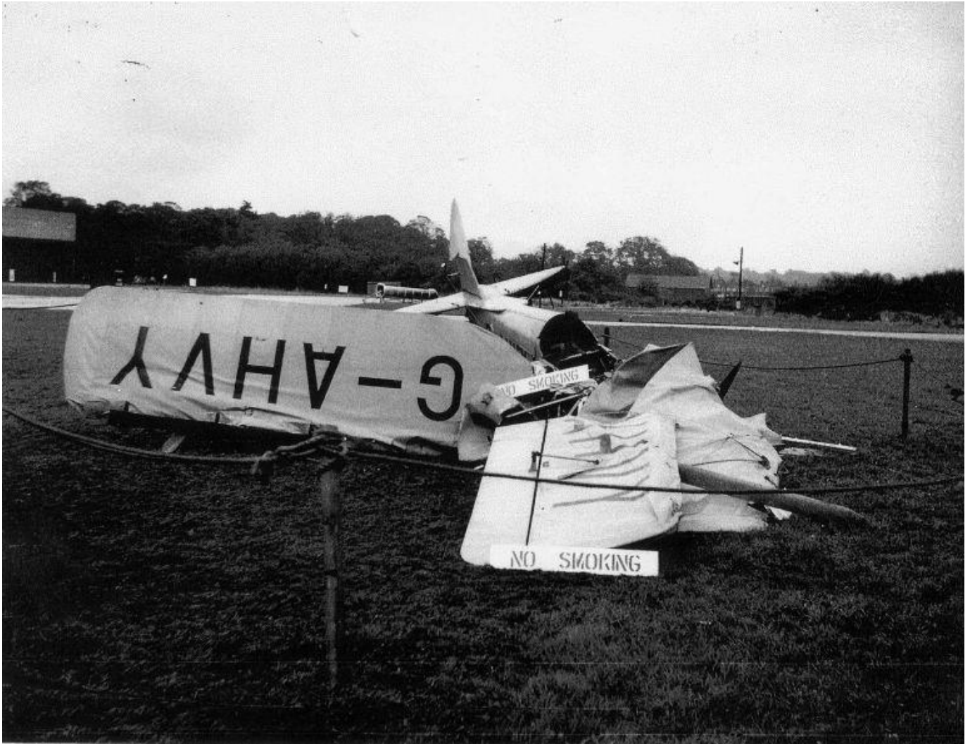
G-AHVY following the fatal crash on 12-11-58 . The control column became detached causing the crash..
