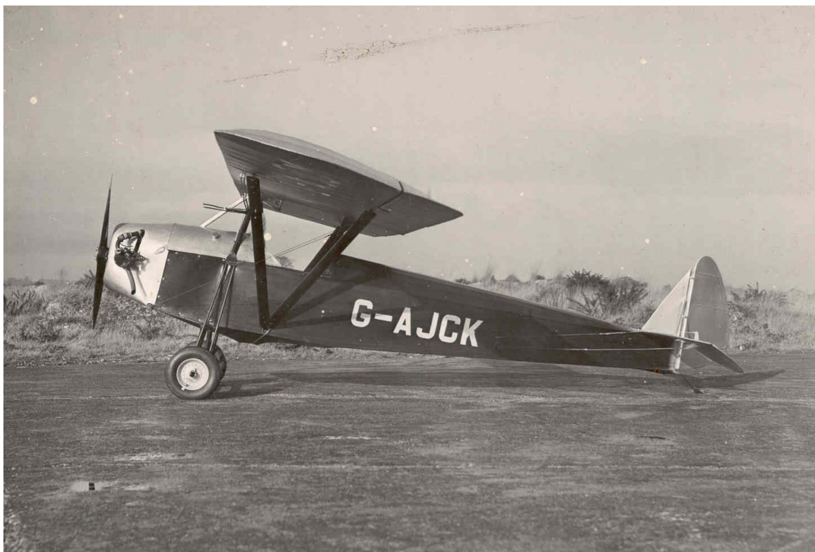
Heath Parasol G-AJCK with ABC engine at Christchurch. The Heath Parasol is an American single-seat, open-cockpit, parasol winged, homebuilt monoplane. During the late 1920s and early 1930s it was the only airplane in the USA that could be constructed at home from a factory-built kit and be licensed by the FAA. Seen below with Ron Clear in cockpit prior to first flight SHULAC secretary Bob Haigh on right.
