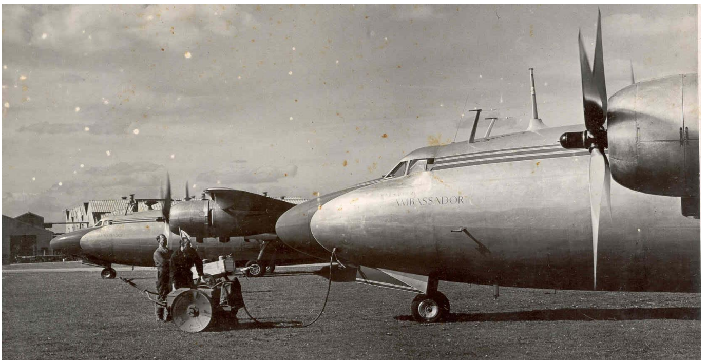
The two prototype Ambassadors being prepared for flight. The second prototype, which was pressurised, is in the background
