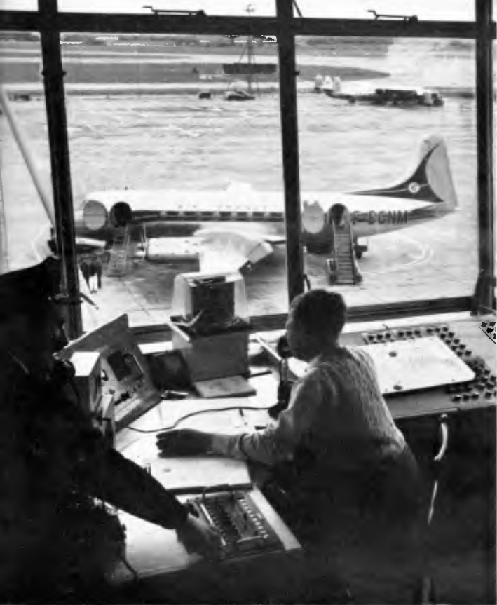
All movement of aircraft on the ground is controlled by a supervisor, who from his station in the Control Tower commands an extensive view over the apron, runways and taxi-tracks
