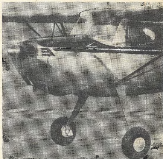
The new Cessna undercarriage showing the unusual thinness of the struts.
