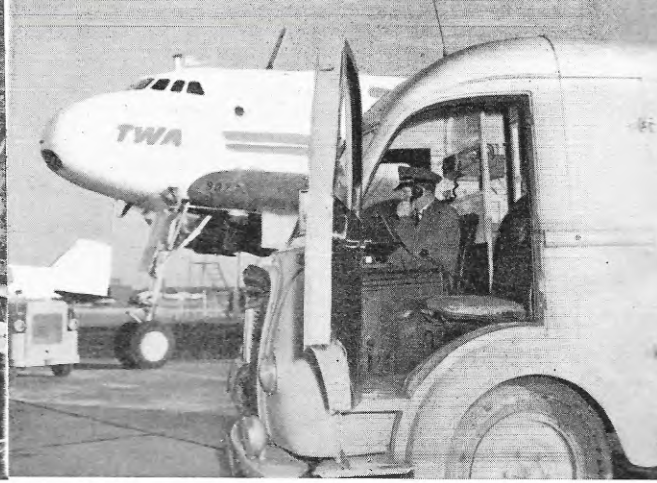
VHF radio-telephones are used extensively to control the movement of servicing and refuelling vehicles.
