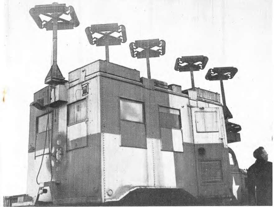
A part of the equipment used to help pilots to land. This is the Localizer Truck of the Instrument Landing System.
