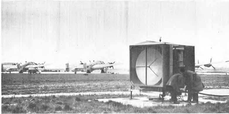
The rotating aerial head of the Airfield Control Radar equipment, which can locate aircraft 25 miles away from London Airport.
